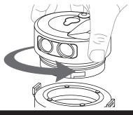
Remove the used Magnesium from the tank.
