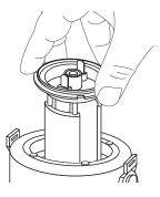
Align  $\square$  mark on the side of the lid with  $\blacktriangle$  mark on the body.Rotate the lid clockwise until align with **A** mark. \*Make sure the lid is sealed well to avoid leakage.
